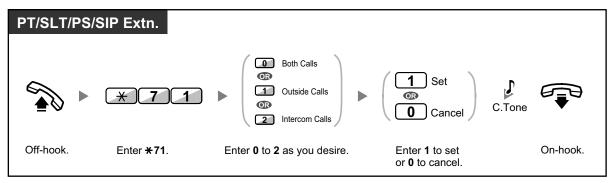
When using a proprietary telephone, you can set or cancel DND by pressing the FWD/DND button (fixed button) instead of "\*710" • The FWD/DND button light shows the current status as follows:
