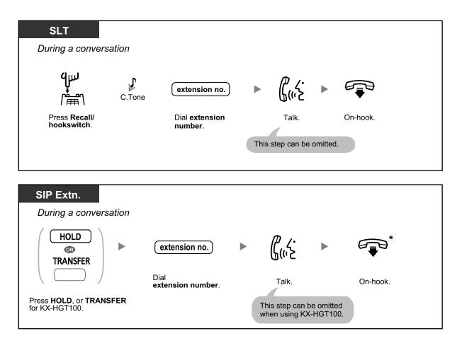
\* Instead of going on-hook, if you press the HOLD button or TRANSFER button (KX-HGT100) once or twice (depending on the telephone being used), you can return to the held call, and the call with the transferred party will be disconnected.
