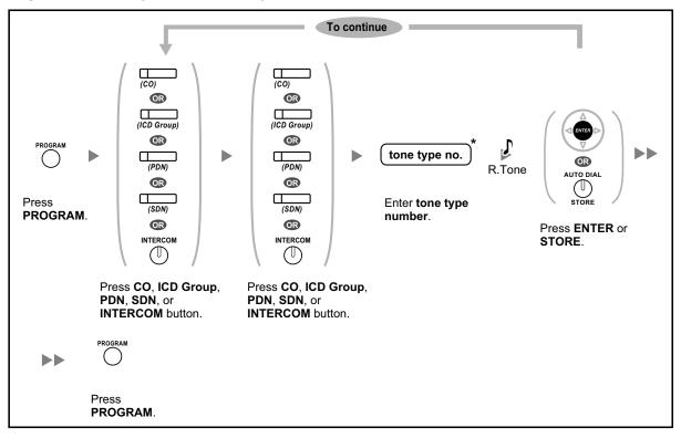
To distinguish the ringing tones for each CO, ICD Group, PDN, SDN, or INTERCOM button (Digital proprietary telephone only)
